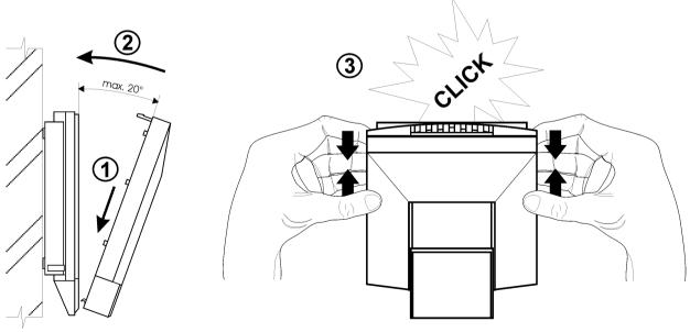
Figure 1: Device mounting
