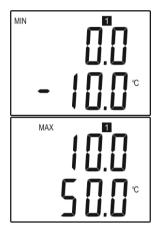
Short button press shows low range and type of measured value for first output (output Uout1, at LCD indicated by symbol "1"). Type of measured value is indicated with appropriated value unit. (here "C = temperature). Upper line shows voltage value which is assigned to value of measured value (lower display line). Here 0 V corresponds with temperature of -10 °C.
