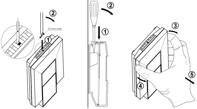
Figure 2: Device demounting
